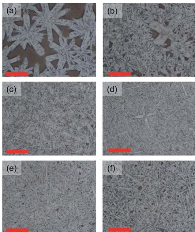
Fig. 1 Optical microscopy images of spray-deposited thin-films of methylammonium iodide and lead chloride onto substrates held at a range of elevated temperatures. (a) 28 °C, (b) 38 °C, (c) 55 °C, (d) 75 °C, (e) 80 °C, (f) 87 °C. The scale bar in each image corresponds to 20 μm.
