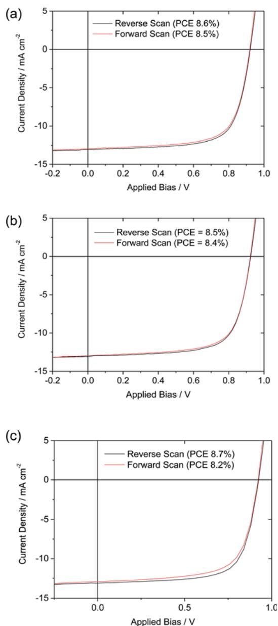
Fig. 4 Current-density versus voltage characteristics for a perovskite solar cell device measured under different scan rates and scan directions: (a) 0.5  $\text{V s}^{-1}$ , (b) 1  $\text{V s}^{-1}$  and (c) 2  $\text{V s}^{-1}$ . Efficiency values are shown in each figure legend. Note that the forward bias sweep conditions reported in part (b) correspond to our standard testing protocol.
